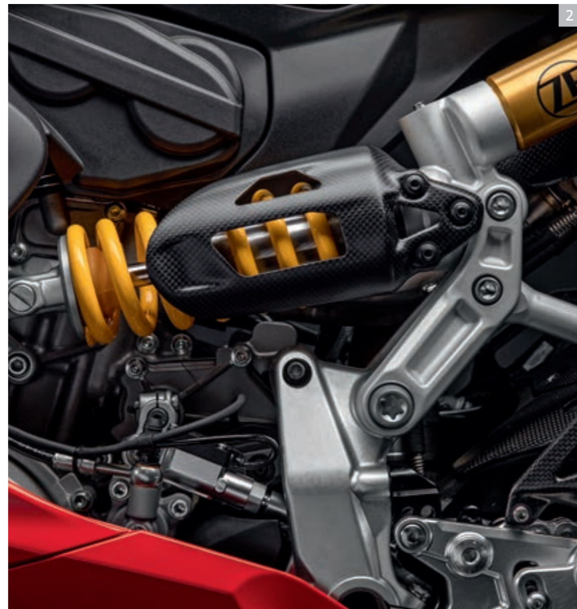
2 Carbon cover for rear shock absorber.
