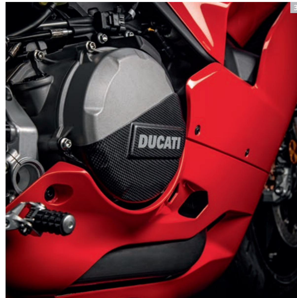
3 Carbon cover for clutch case.
