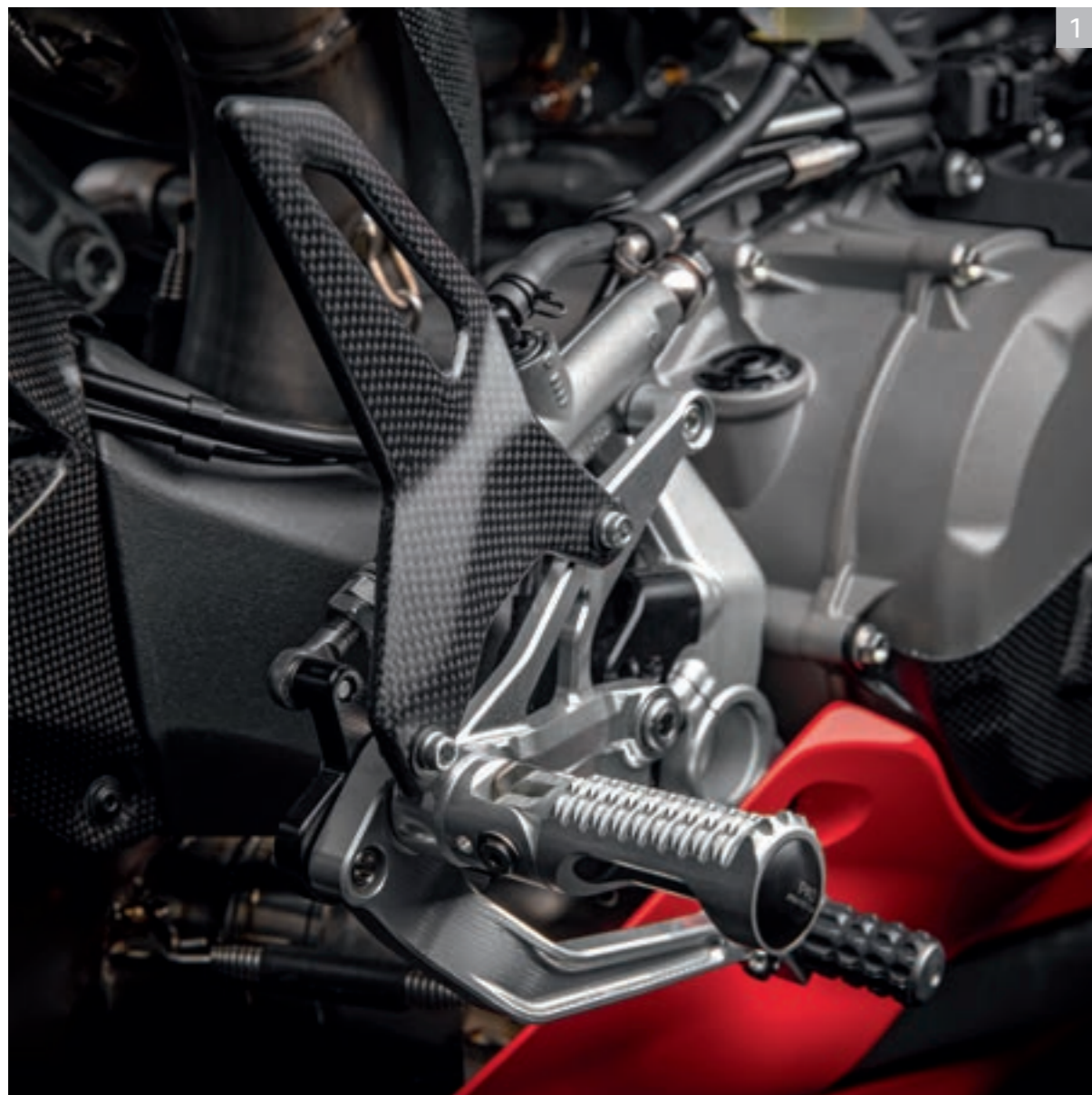
1 Carbon heel guard. Adjustable rider footpegs in aluminium.
